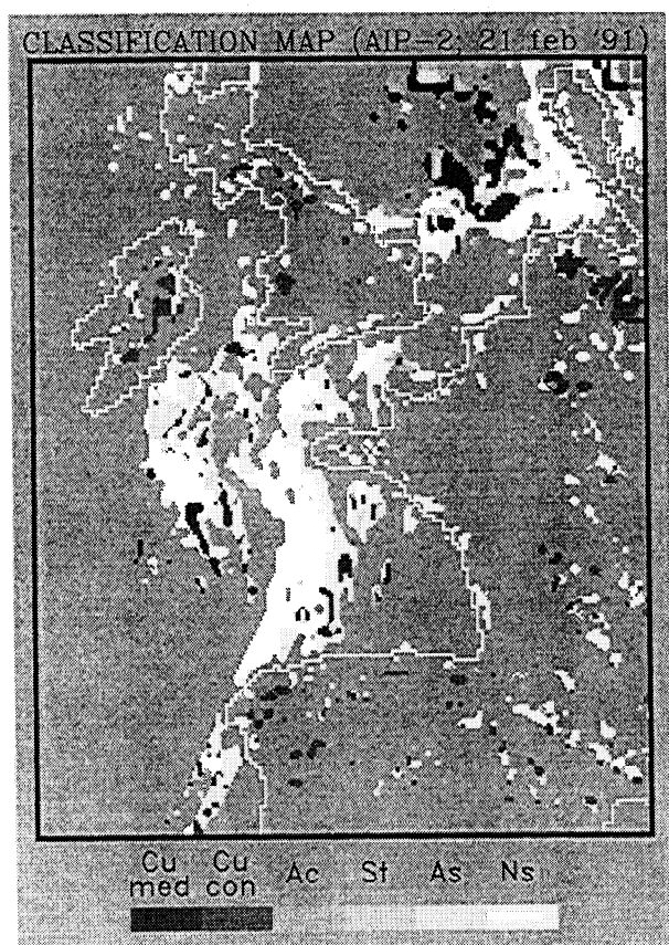
Figure 12. Cloud genera map derived from SSM/I data acquired on February 21, 1991, at 0837 UTC by applying the maximum-likelihood (ML) classification algorithm after discriminating the cloud coverage, as explained in the text.
