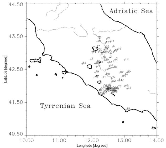
Fig. 1. Rain gauge network of the Tiber River basin. The location of each station is indicated by a cross and the index ranges from 1 to 86 (the maximum number of active rain gauges).
