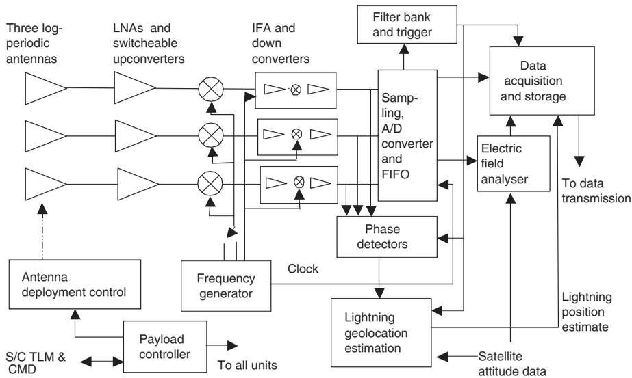
Figure 2. Single-satellite system payload block diagram. LNA, low noise amplifier; S/C, spacecraft; TLM, telemetry; CMD, command; IFA, intermediate frequency amplifier; and A/D, analogue to digital.
