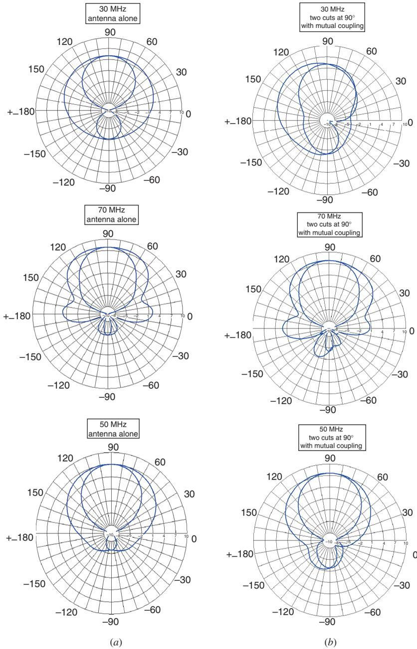
Figure 4. Antenna patterns (a) without mutual coupling and (b) with mutual coupling.
