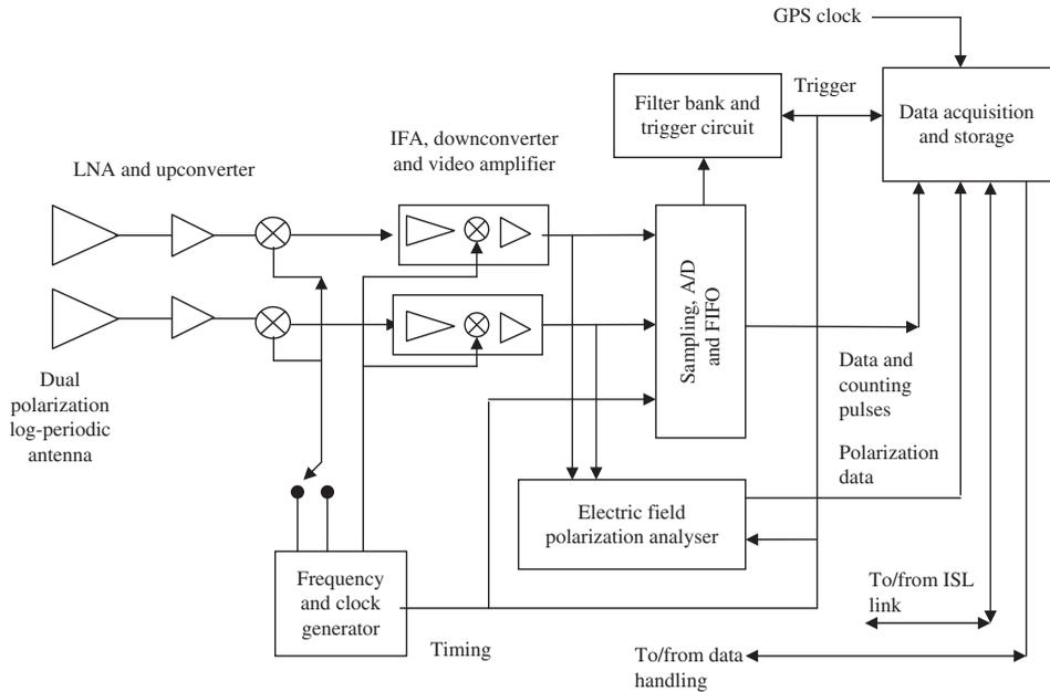
Figure 5. TOA-based constellation: payload block diagram.
